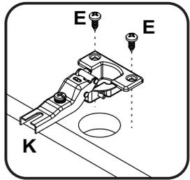
**A** Cavilha **04** **E** Parafuso  $\varnothing 4,0 \times 14 \text{mm}$  CP **04** **K** Kit Dobradiça Ata **02**
