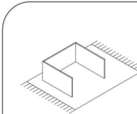
**The module must be mounted above soft surface, such as a carpet.**
