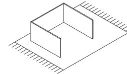
**The module must be mounted above soft surface, such as a carpet.**
