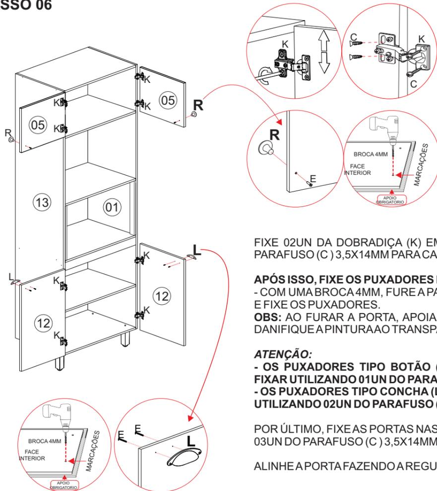
FIXE 02UN DA DOBRADIÇA (K) EM CADA PORTA (05, 12), UTILIZANDO 03UN DO PARAFUSO (C) 3,5X14MM PARA CADA UMA.
