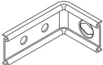
CANTONEIRA METALICA PARA FIXAÇÃO NA PAREDE | <b>4</b>   | <b>J</b>
