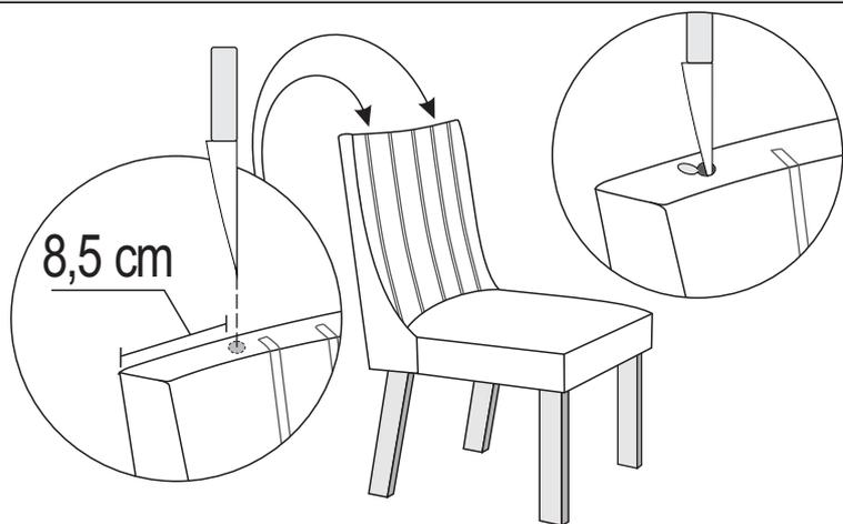
**4º** - PASSE COLA NOS FUCOS DOS DETALHES E COLOQUE AS CAVILHAS E BATE LEVEMENTE COM UM MARTELO DE BORRACHA ATÉ ENCAIXAR AS CAVILHAS NOS DETALHES.
