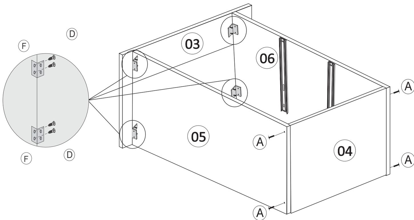
09=FIXE A BASE ( 04 ) NOS PES SUPERIORES ( 10 ) COM PARAFUSO ( A )
