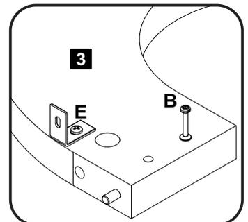
**A** Cavilha 04 **B** Minifix Ø7x30mm 12 **E** Parafuso Ø4,0x14mm CP 04 **H** Cantoneira 1"x1" 04 **K** Sapata 04
